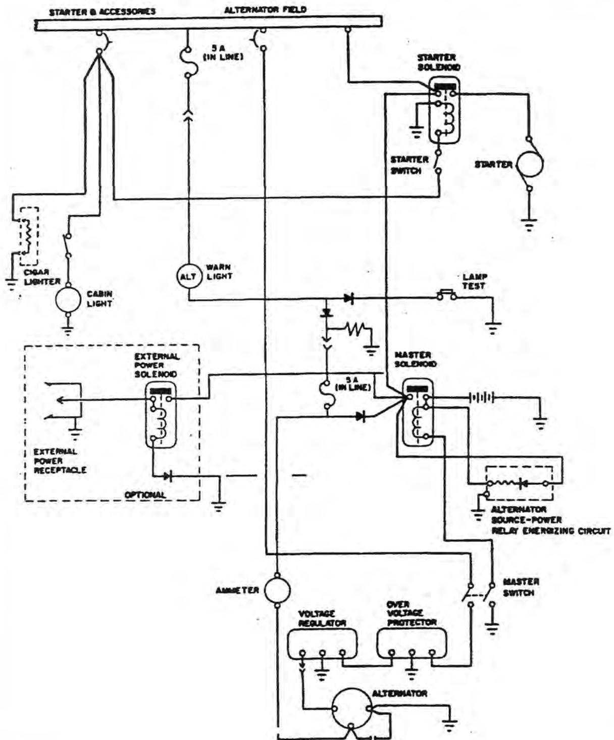
ALTERNATOR AND STARTER SCHEMATIC
