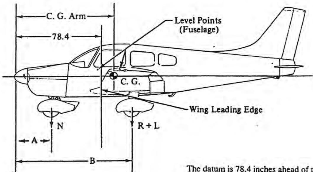
The datum is 78.4 inches ahead of the wing leading edge at the intersection of the straight and tapered section.
